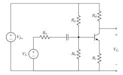
2. In the following circuit, assuming  $\beta \approx Beta$  and that  $V_{be} \approx 0.65V$ , find the value of  $R_g$  such that the DC level of  $V_{f_o}$  is equal to DC level.
